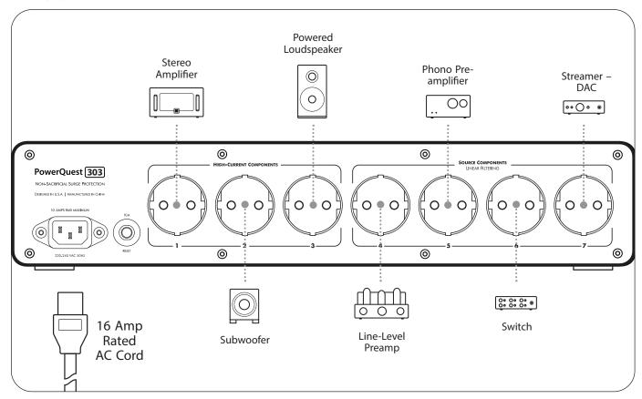
**Note:** Outlets 4 through 7 are subject to many variables and circuit conditions, so experimentation for best results is encouraged. Power amplifiers must be connected to outlets 1 through 3.
